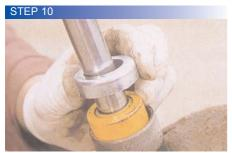
Slide your smart new uprated damper into the strut the right way. Carefully spin on the collar and tighten with your peg scanner
