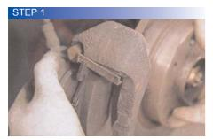
Unscrew the two large bolts that hold the brake caliper to the wheel hub. Remove the bolts and move the caliper out of the way. Don't let it dangle!
