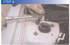
The strut is almost ready to come out. Under the bonnet you'll see where the strut bolts to the body. Undo the bolts and it will fall out easier than a ho's tit
