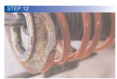
Refit the rubber dust boot, and make sure the springs sits in its lower cup. Slide on the upper cup and strut top before tightening up the top mount nut
