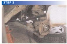
The bottom of the struts is held onto the suspension arm with a pinch bolt. Remove the bolt. You may need a crowbar to prise the two apart
