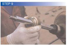
The damper's hidden inside the strut. Using a peg spanner, undo the collar that holds the damper in the strut. Don't damage it. Pull out the old insert
