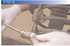
Now you fit the spring clamps, one on each side as shown. If not, when you take the strut apart, the coil will fire out and smack you in the face
