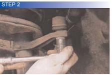
The steering arm is connected to the strut with a balljoint. With a socket, undo it and pop the balljoint out. You may need a balljoint splitter to help here
