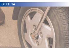
Refit the brake disc and caliper. Fit the wheel and drop the car back. Tighten the drive-shaft/disc nut to the recommended torque setting
