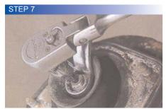
Undo the top mount nut while holding the damper shaft with an Allen key. Pull off the top mount bearing and plates, noting their order
